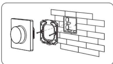
Fix the controller base on the bottom case with screw.
